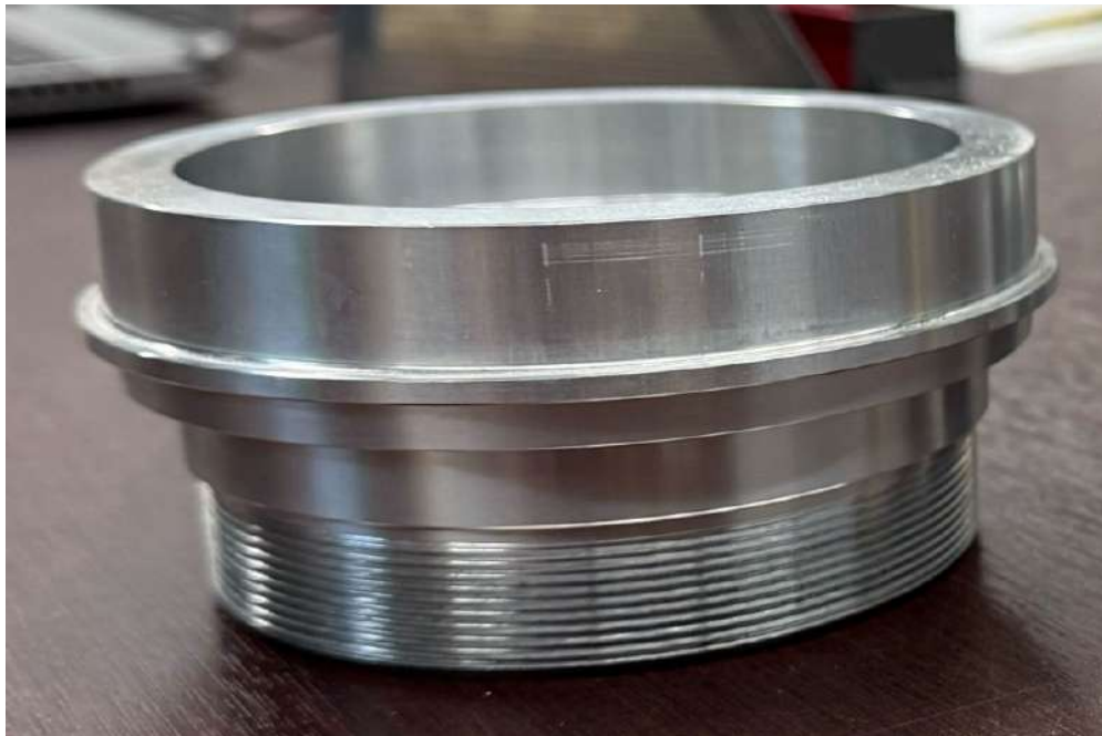
Figure 1J: Partially manufactured thrust plate.
